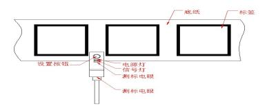
4, Pass labels through the Magic Eye's U the slot, as shown in the following illustration.
