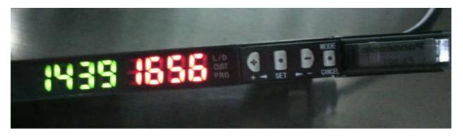
5.2.2.2 The principle of measuring the electric eye detection: The electric eye of a substance is a that identifies an object according to light reflection. The electric eye emits light to the object, the object will reflect a certain amount of light back to the eyes, when the object reflects the amount of light reached the set value, the Magic eye signal changes, signal to the control system.
